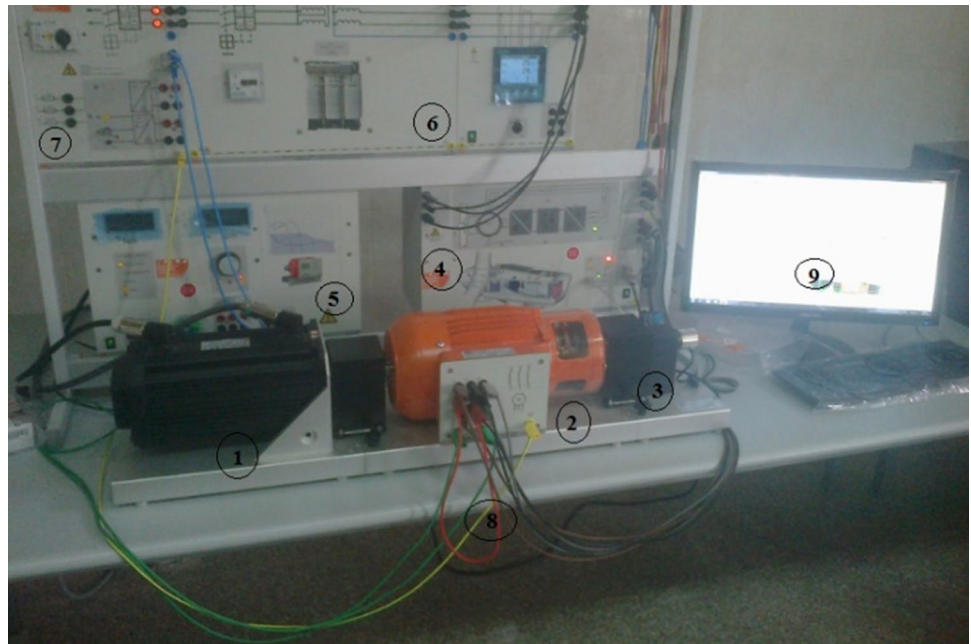
Fig. 10 Hardware used to co-simulate of a DFIG-based wind turbine. 1. Servo motor, 2. DFIG, 3. Encoder, 4. DFIG control unit, 5. Servo control unit, 6. Three-phase transformer, 7. Grid unit, 8. Wiring connection, and 9. PC control unit.
