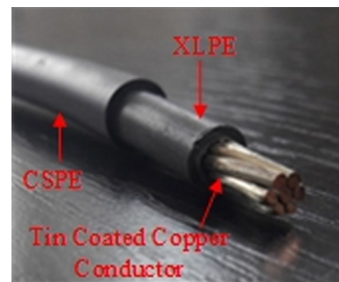
Fig. 1. Low-voltage power cable sample under investigation
