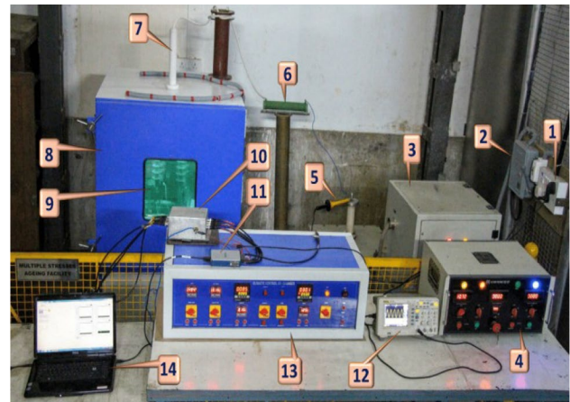
Fig. 1 Developed multistress aging facility. 1: AC 230 Volt, 50 Hz power supply, 2: 400 Volt, 50 Hz power supply, 3: HVAC source, 4: HVAC control panel, 5: high-voltage probe, 6: current-limiting resistor 15 k \Omega , 500 W, 7: high-voltage bushing, 8: aging chamber, 9: UV-protected glass, 10: shunt box, 11: NI cDAQ for LC measurement, 12: digital oscilloscope, 13: climate chamber control panel, 14: NI cDAQ data acquisition in LabVIEW environment
