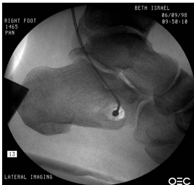
Fig. 1. Fluoroscopic lateral image of a cadaver foot showing the temperature probe implanted in the calcaneus near the tarsal sinus.
