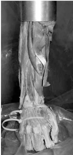
Fig. 4 Fall simulation of the intact arm, which was positioned on a wedge, with 80° pronation and 70° dorsiflection of the hand. The load was applied through the elbow, which was allowed to rotate during the test
