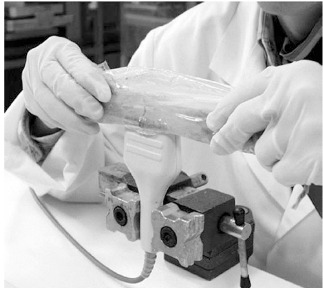
Fig. 2 Acquisition of cortical SOS in the isolated radius. The radius was sealed in airtight plastic bags and scanned with an Omnisense 7000 scanner (Sunlight Medical) at 33% radius length
