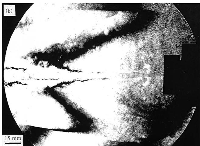
Fig. 6a,b. Interferogram of 2 km/s diesel fuel jet from a 2.5 mm diameter nozzle. Chamber pressure and gas: 3.26 MPa air
