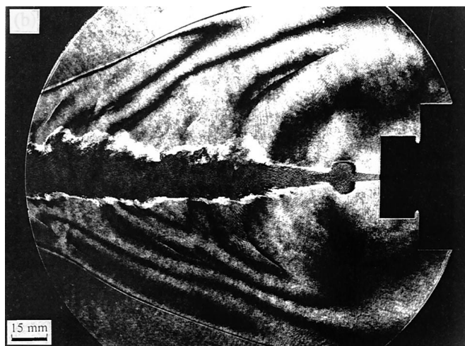
Fig. 7. Interferogram of 2 km/s diesel fuel jet from a 2.5 mm diameter nozzle. Chamber pressure and gas: 0.1 MPa in helium/air
