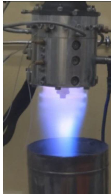
Fig. 4 Combustion chamber and the exhaust
