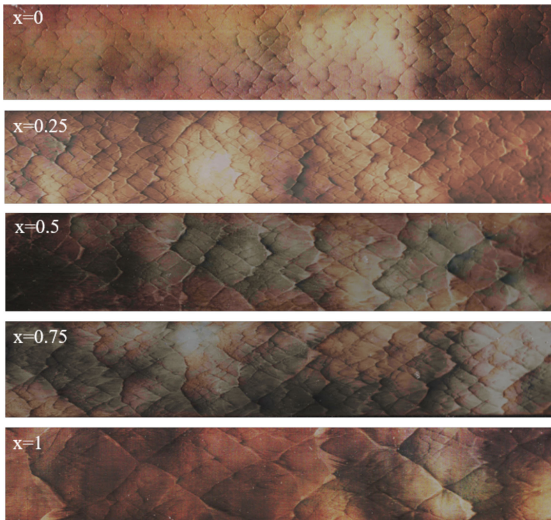
Fig. 3 Upstream soot-foil recordings showing the detonation cellular structure depending on the composition x of the mixtures (1-x)\text{H}_2 + x\text{CH}_4 + 1/2(1+3x)\text{O}_2 at initial pressure p_0 = 25 kPa
