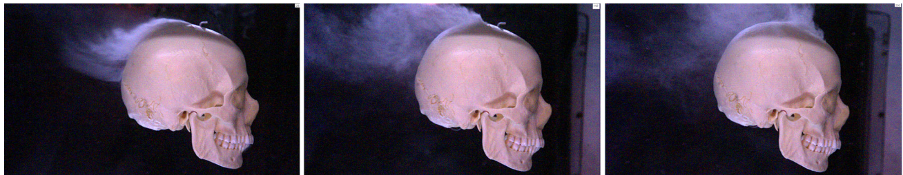
Fig. 11 Visualization of the blast-wave flow around a replica skull head-form at 1.0 and 5.7 (onset of negative phase) and 8 ms after shock arrival
