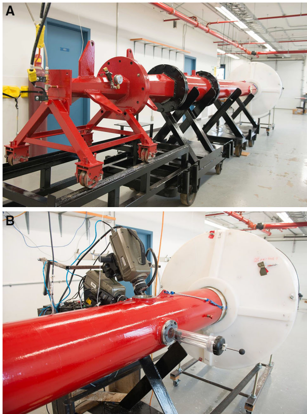
Fig. 1 Advanced blast simulator (ABS). The ABS consists of a divergent driver (foreground, a ) separated from a transition section by a frangible diaphragm. The transition section leads to the ambient-pressure test section. The ABS is 5.79 m in length with a circular test section diameter of 30.5 cm, b the test sample port where the clear cylindrical animal restraint device is placed, as well as the end wave eliminator (EWE) that prevents rarefaction waves from re-entering the test section. Also depicted is the positioning of the high-speed cameras that view test samples through two polycarbonate window ports
