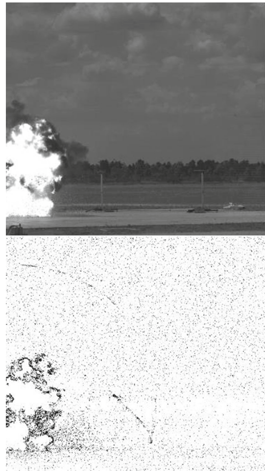
Fig. 4 Focused camera view 7.3 ms after the detonation of the 500 g charge at 133 cm. (Top) raw camera data, i.e., single frame. (Bottom) difference between two consecutive frames
