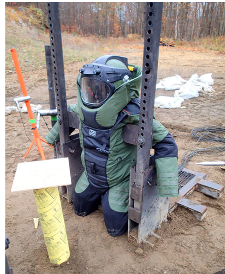
Fig. 3 Hybrid III mannequin held in a kneeling position (explosive ordnance disposal ensemble)
