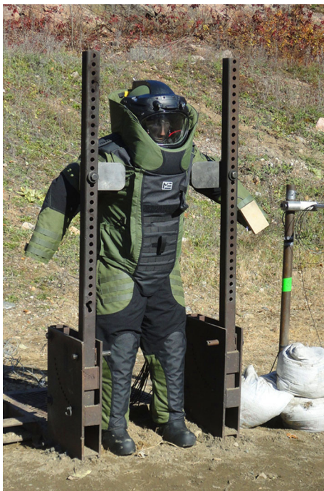
Fig. 2 Hybrid III mannequin held in a standing position (explosive ordnance disposal ensemble)
