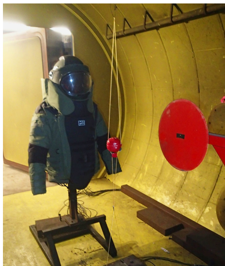
Fig. 7 Indoor blast chamber test example (CERL, Ottawa, Canada) with an explosive ordnance disposal ensemble
