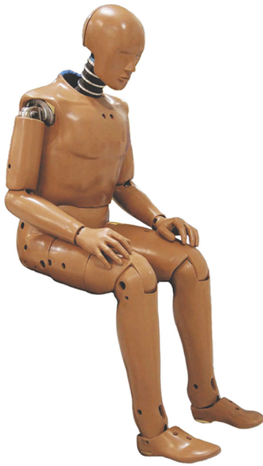
Fig. 1 Hybrid III anthropomorphic mannequin used for blast testing. Humanetics ATD, Huron, OH, USA
