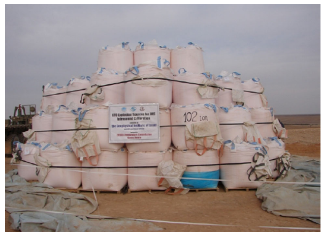
Fig. 1 Experimental charge geometry. Charge consists of four layers of ANFO bags bounded with a steel band for charge compactness and stability. This photograph is reprinted from Fig. 1 of [12] with permission from Springer
