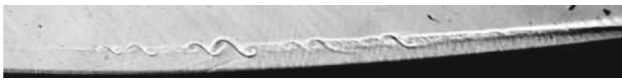
Fig. 1 Experimental images of the Kelvin–Helmholtz instability in a Mach reflection off a curved surface M = 1.5 [6]
