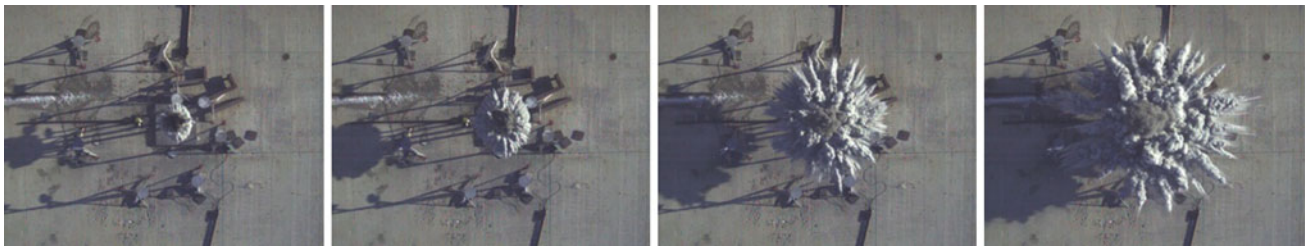
Fig. 1 Explosive dispersal of a 2L cylindrical charge that consists of a small cylindrical C4 explosive packed in a central glass tube surrounded by an annulus of atomized dry aluminum particles [4]
