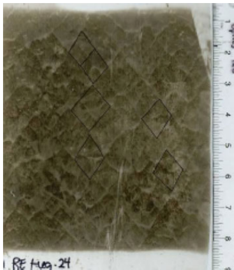
Fig. 3 Typical cell size sample from smoke foil for methanol–oxygen mixture ( p_0 = 10.7 kPa, \phi = 1.0 )
