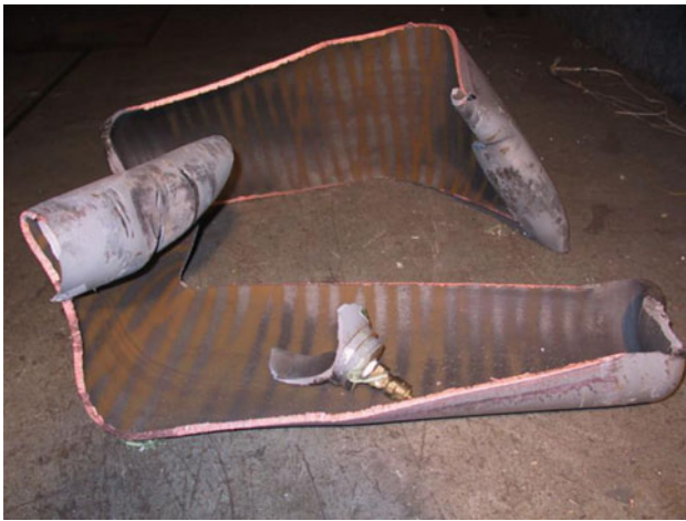
Fig. 5 Typical remains of the CO 2 bottle (experiment 1)
