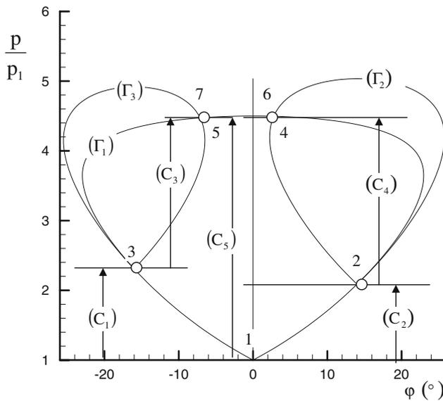
**Fig. 15** Shock reflection with singular shock intersection or Mach phenomenon: Situation in the shock polar plane ( $M_1 = 2$ ,  $\varphi_1 = 14^\circ$ ,  $\varphi_2 = -16^\circ$ )
