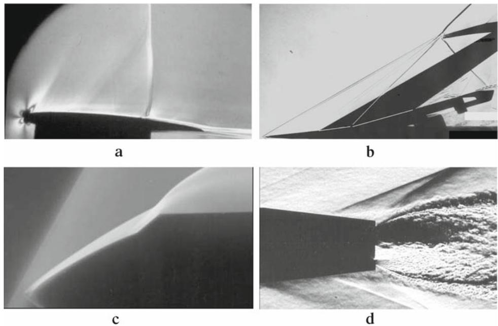
**Fig. 2** Basic shock wave/boundary layer interactions (Onera documents). **a** oblique shock reflection, **b** ramp induced shock wave, **c** normal shock wave, **d** adaptation shock at a nozzle exit
