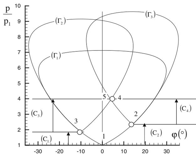
**Fig. 13** Shock pattern interpretation in the shock polar diagram. Upstream Mach number 2. Separation shock deflection  $14^\circ$ ; incident shock deflection  $-10^\circ$
