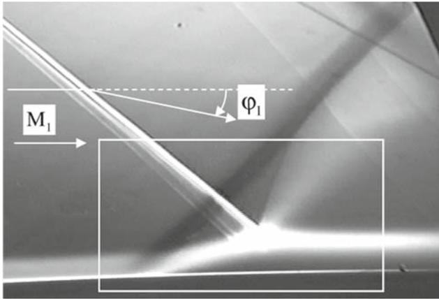
**Fig. 10** Schlieren visualisation of an incident-reflecting shock at Mach 2 (Onera document)
