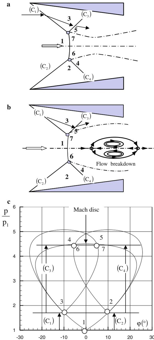
**Fig. 17** Direct and inverse Mach phenomenon. **a** direct Mach phenomenon, **b** inverse Mach phenomenon, **c** inverse Mach phenomenon: Situation in the shock polar plane ( $M_1 = 2$ ,  $\varphi_1 = 10^\circ$ ,  $\varphi_2 = -10^\circ$ )
