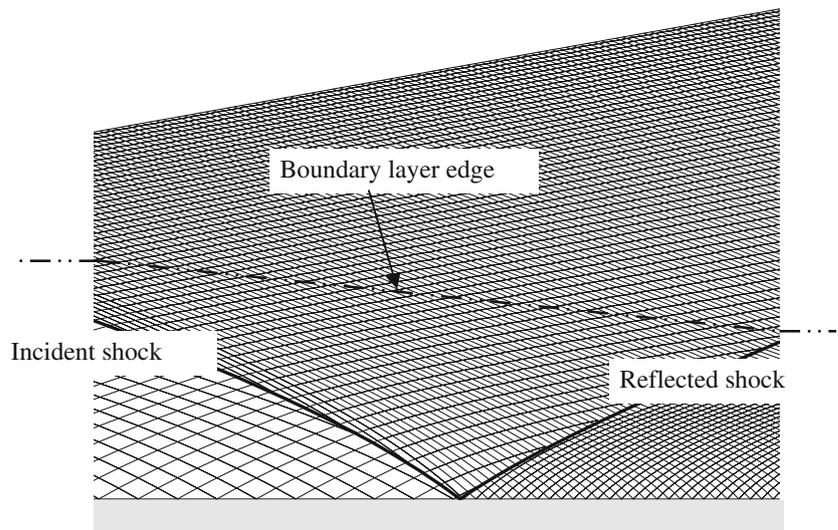
**Fig. 8** Method of characteristic calculation of a shock reflection in a rotational layer. Entropy gradient effect on the wall pressure distribution (upstream Mach number 4- primary deflection  $6^\circ$ )
