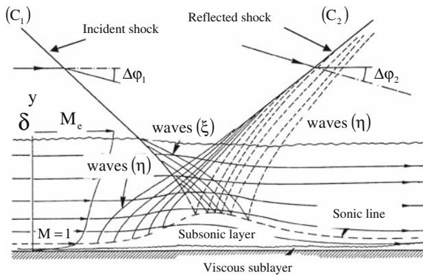
**Fig. 5** A sketch of a turbulent shock reflection without boundary layer separation
