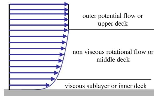
**Fig. 3** The interacting flow multi-layer structure or triple deck (Lighthill, Stewartson–Williams)
