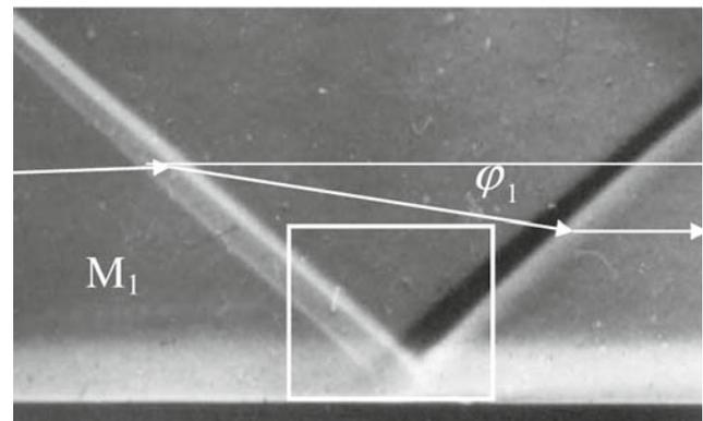
**Fig. 4** Schlieren photograph of a shock reflection at Mach 1.95 (Onera document)
