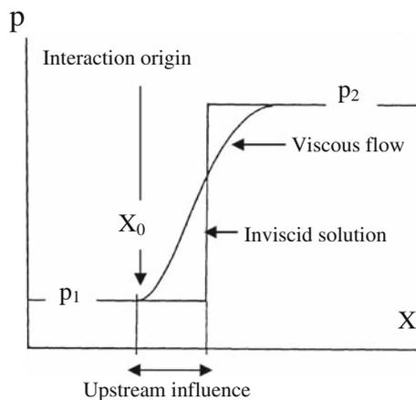
**Fig. 6** The corresponding pressure distribution
