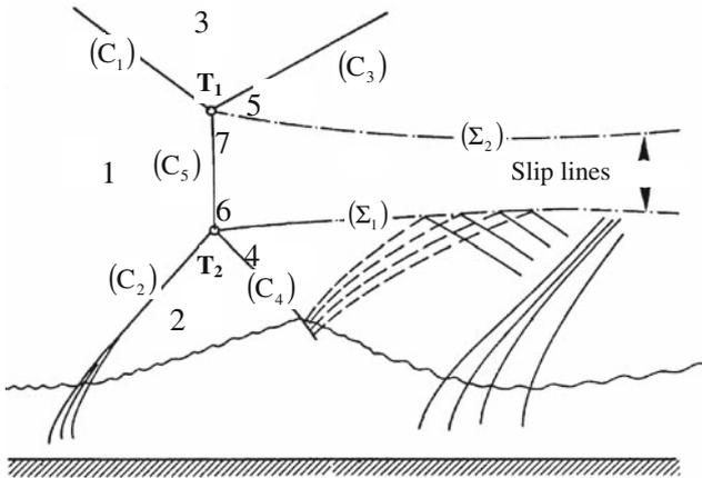
**Fig. 14** Shock reflection with singular shock intersection or Mach phenomenon: Schematic view of the situation in the physical plane
