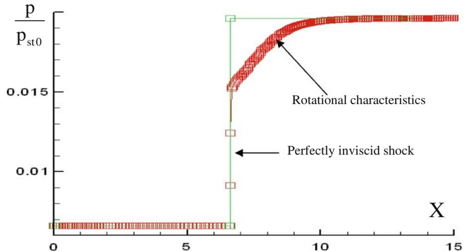
description of the complex wave pattern which is generated when a shock traverses a boundary layer considered as a rotational inviscid stream. However, the above scenario does not take into account the upstream transmission through the subsonic part of the boundary layer with the subsequent generation of compression waves, which coalesce to produce the reflected shock.
