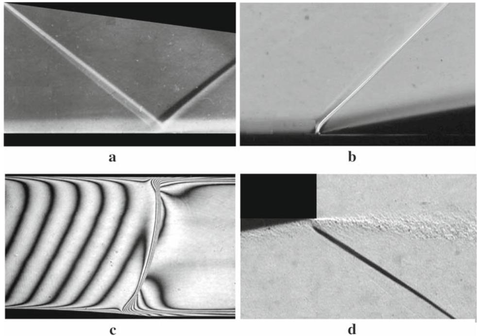
a supersonic air-intake of the mixed compression type or at the impact of the shock generated by any obstacle on a nearby surface.
