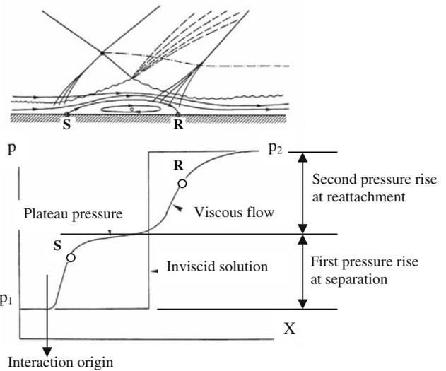
**Fig. 12** Wall pressure distribution, in a shock separated flow
