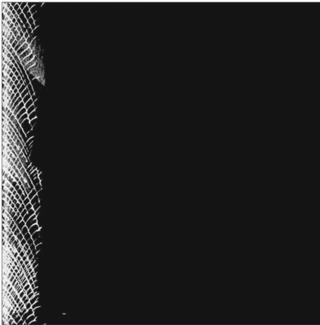
Fig. 12 Smoke-foil record written by triple shocks in rotating detonation after t = 6,250\mu\text{s} (during steady rotation), where white lines are trajectories of pressure higher than 6 MPa during detonation propagation. Cell size is 3–3.5 mm near injection wall, while 4 mm in downstream side
