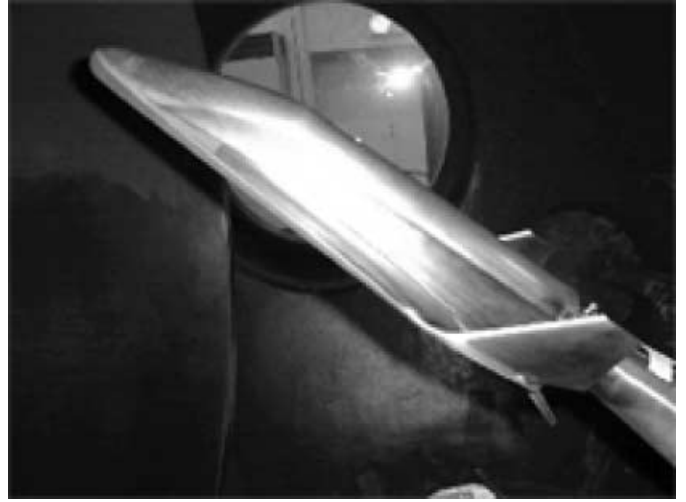
Fig. 2. 2.5% HOPE model equipped with force balance
