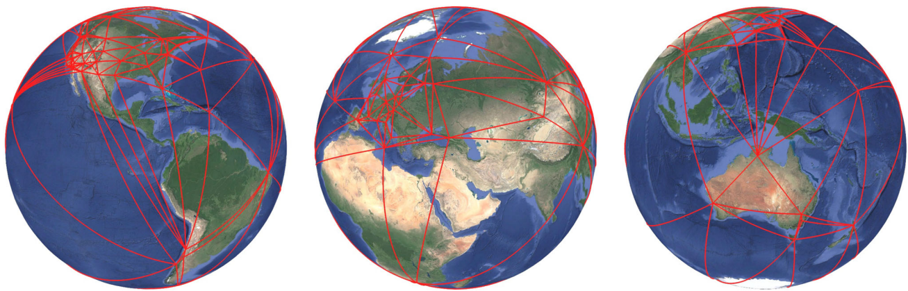
Fig. 16 The Delaunay triangulation of the ITRF14-VLBI (2016) dataset (radio telescopes)—a global surface mesh of 304 triangles with areas between 0.5 ha and 27.4 mil. km 2 ; the average triangle side length is 1450 km, and the average triangle area is 1399,682 km 2
