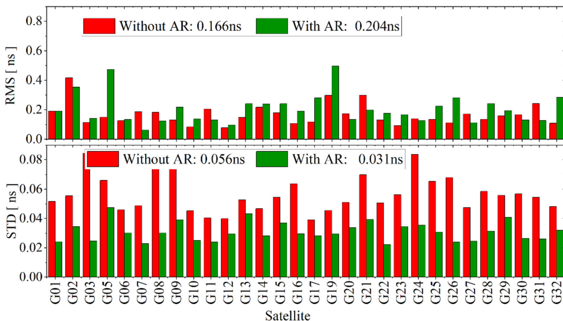
Fig. 10 Averaged RMS and STD of GPS satellite clock between filter solution and IGS final products
