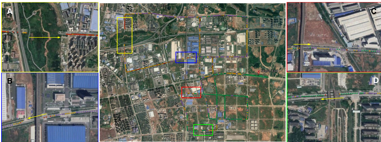
Fig. 13 Field test in urban environment. The trajectory is from GPS-alone PPP solutions. Different colors on the trajectory correspond to different number of satellites. Red represents n \leq 5 , yellow represents n
