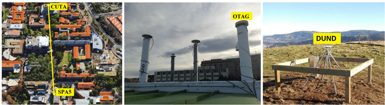
Fig. 9 GNSS Trimble NetR9 receivers collecting data for GPS + BDS single-baseline (ionosphere-fixed) RTK, involving CUTA-SPA5 (350 m baseline, May 14–15, 2015) in Perth ( left ) obtained through Map data
