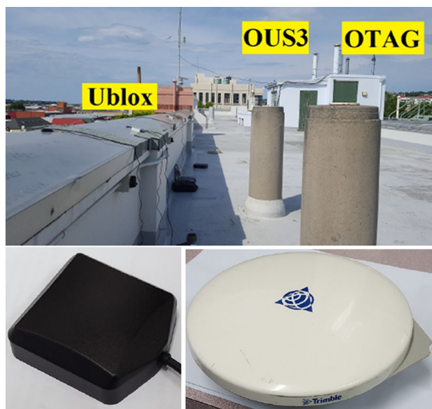
Fig. 13 Low-cost single-frequency ublox EVK-M8T GNSS receivers (top) with patch antennas (bottom left) collecting data for L1 GPS + B1 BDS single-baseline (ionosphere-fixed) RTK (November 25, 2015) in Dunedin. The survey-grade multiple-frequency receivers (top) OTAG (Trimble NetR9) and OUS3 (Septentrio PolarX4) are connected to choke-ring antennas. Four days later (November 29, 2015) the ublox receivers were collecting data with the same GPS and IGSO/GEO constellation repeated, but then connected to Trimble Zephyr 2 antenna (bottom right)
