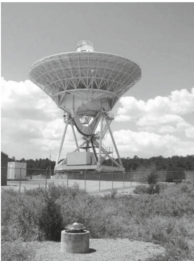
Fig. 2 The VLBA station PIETOWN is in the background. The permanent GPS receiver PIE1 is in the foreground
