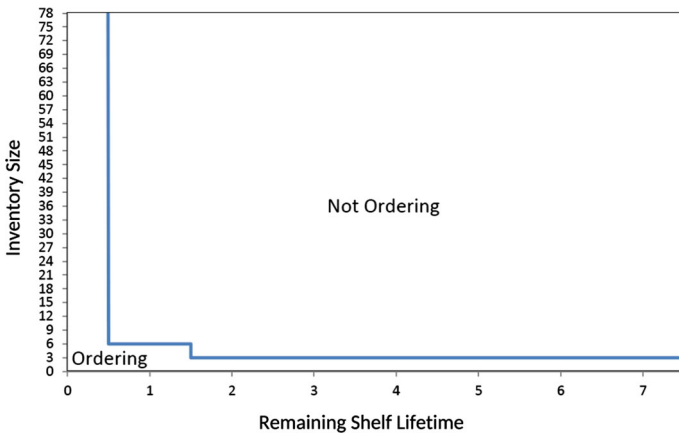
Fig. 4 Optimal decision policy structure for any inventory size and remaining shelf lifetime
