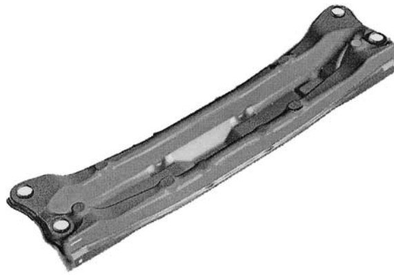
Fig. 4. Production model of the rear bridge.
