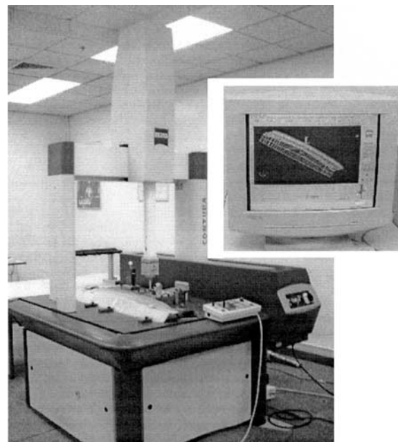
Fig. 4. Digitised measurement by CMM.
