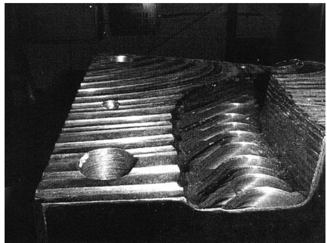
Fig. 6. 3-Axis contour rough machined die insert.
