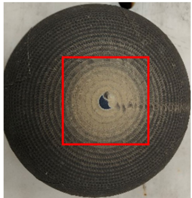
Fig. 4 Actual effect of machining at a constant feed rate
