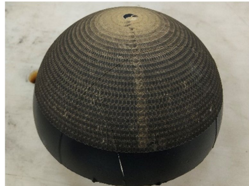
Fig. 10 Effect of constant feed rate machining of nickel alloy spherical shells
