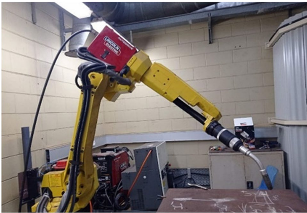
Fig. 2 The FANUC welding robot set-up used in the experiment
