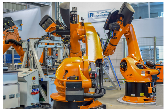
Fig. 2 Forming setup at the chair of production systems (LPS). The forming experiments were carried out by two KUKA KR600 robots, each driven by KRC4 controller (background)[23]
