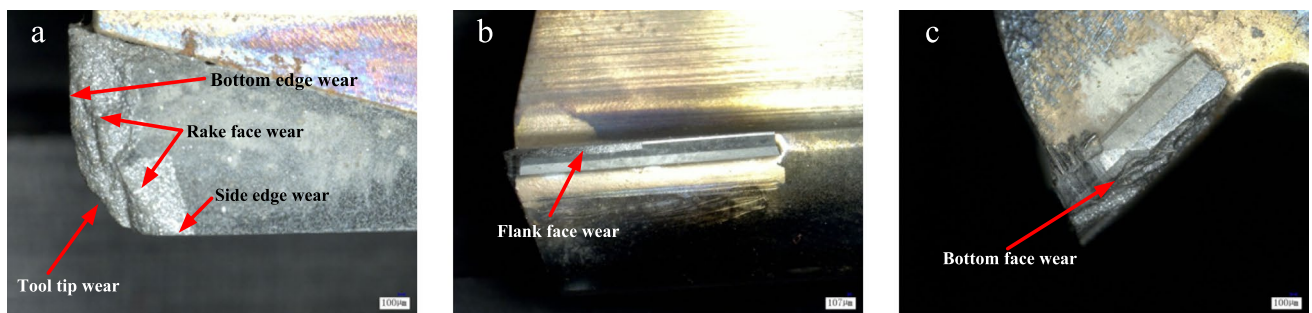
Fig. 17 Tool surfaces, worn tool. (a. rake face 50×; b. flank face 20×; c. bottom face 50×)
