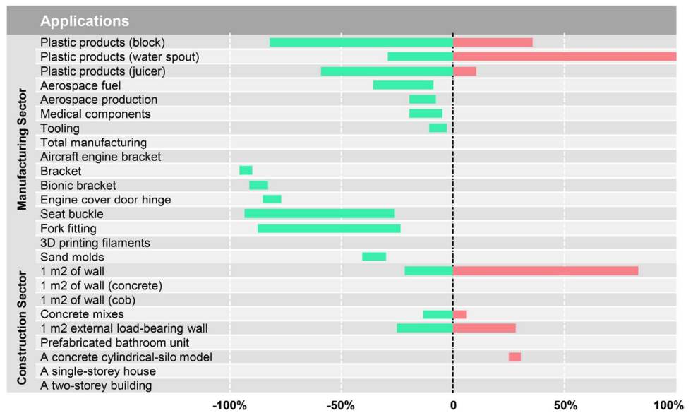
Fig. 8 Summary of available studies estimating greenhouse gas (GHG) emissions of 3D printed products in manufacturing and construction compared to traditionally manufactured counterparts. Reprinted and adapted from [107] with permission from Elsevier
