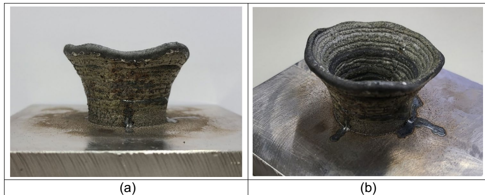
Fig. 19 Image of first toolpath experiment: a front view and b top view
