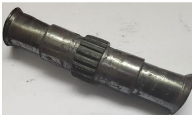
Fig. 17 Finished product of the cross wedge rolling experiment
