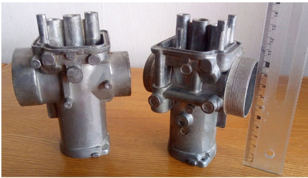
Fig. 5 Carburetor housings made by the optimal HPDCP
