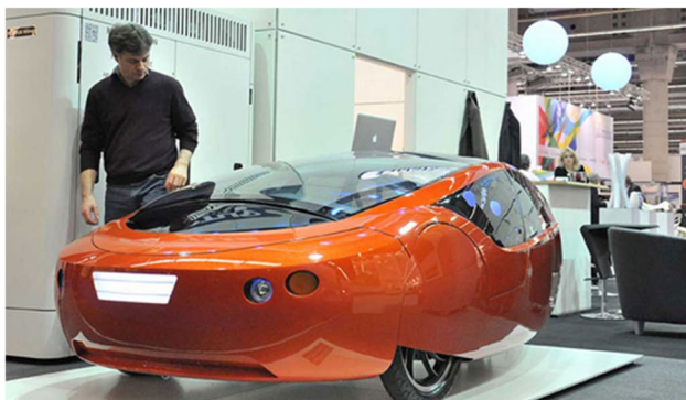
Fig. 23 First energy-efficient automobile vehicle printed with FDM [214]
