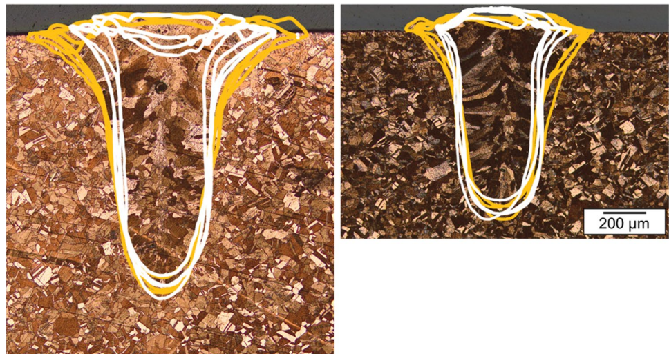
Fig. 12 Superimposed seam contours for varied beam profiles (orange contour, EL; white contour, TH) and equal penetration depth; \lambda=515 nm, P=2.5 kW (EL)/2 kW (TH), v=8 m/min (left); P=2.5 kW (EL)/2 kW (TH), v=18 m/min (right)
