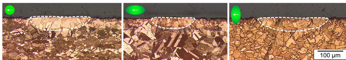
Fig. 9 Weld seam cross sections for varied beam profiles TH (left), EL (middle), and EL,90° (right) and indicated remelted area; \lambda = 515 nm, P = 0.5 kW, v = 4 m/min, feed direction indicated by white arrow
