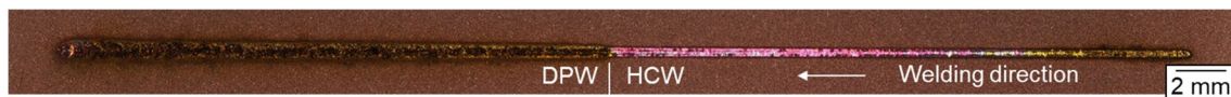
Fig. 8 Top view of weld seam with increased laser power for constant feed rate: transition from HCW to DPW; beam profile EL,90°, \lambda = 515 nm, P = varied, and v = 8 m/min
