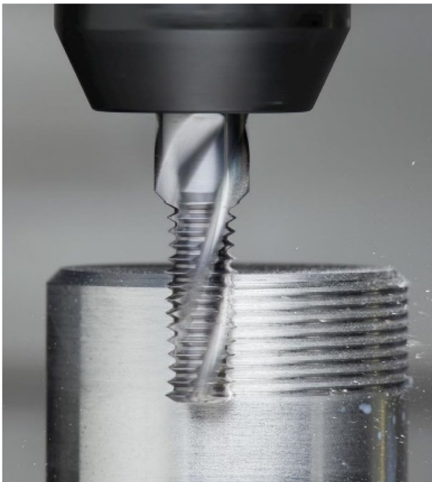
Fig. 3 External thread milling with a multi-form cutter
