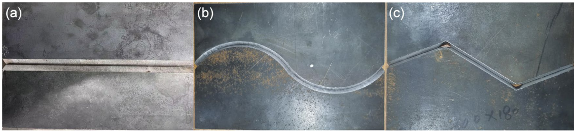
Fig. 13 Experimental workpieces of a straight, b curved, and c folded types
