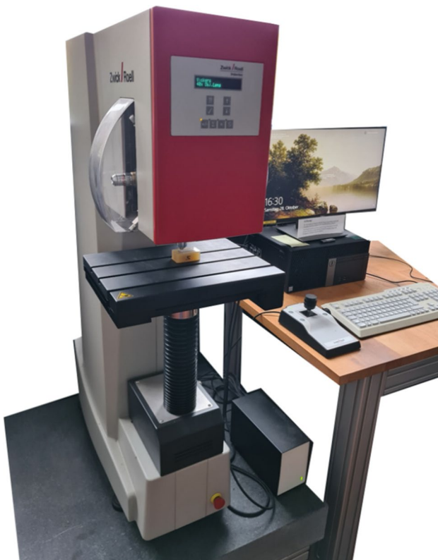
Fig. 8 Universal hardness testing machine ZHV30
