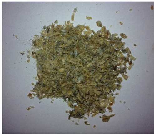
Fig. 2 Composite sample prepared for TGA
