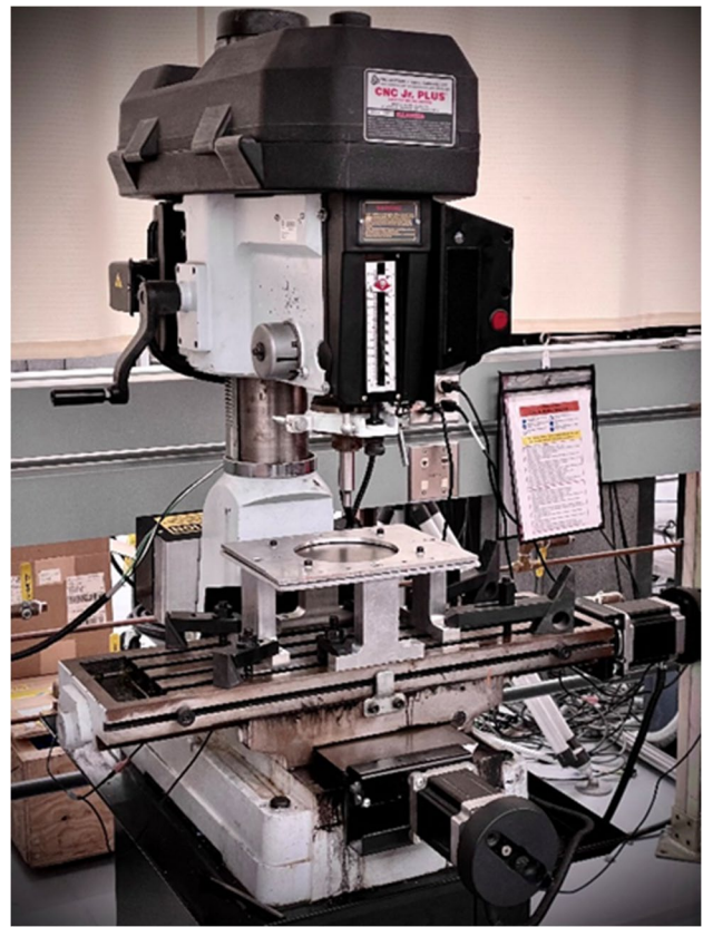
Fig. 2 SPIF setup implemented on a benchtop CNC milling machine
