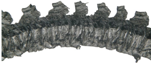
Fig. 4 Back side of the chip produced at a cutting speed of 150 m/min and a feed rate of 0.15 mm/rev
