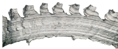
Fig. 3 Front side of the chip produced at a cutting speed of 150 m/min and a feed rate of 0.15 mm/rev
