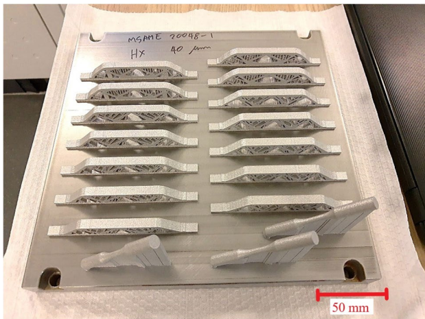
Fig. 11 Printed tensile and optimized beam samples. Note that only 3 repeats of the tensile dogbone samples inclined at 45° are shown in this figure. Other orientations described in Fig. 10 were printed in other build beds that are not shown
