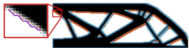
Fig. 4 Nodes in orange showing overhanging edges for the optimized topology in Fig. 3. The enlarged region shows an edge connection made in purple
