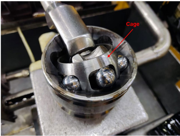
Fig. 1 Automotive cage housing ball bearings—part of a constant velocity joint (CV joint)—which transfers torque from the motor to the drive wheels
