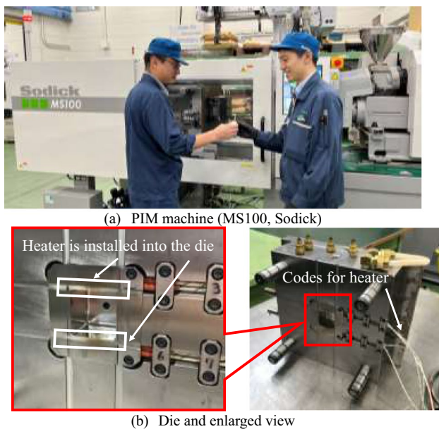
Fig. 14 PIM machine (MS100, Sodick), die and enlarged view
