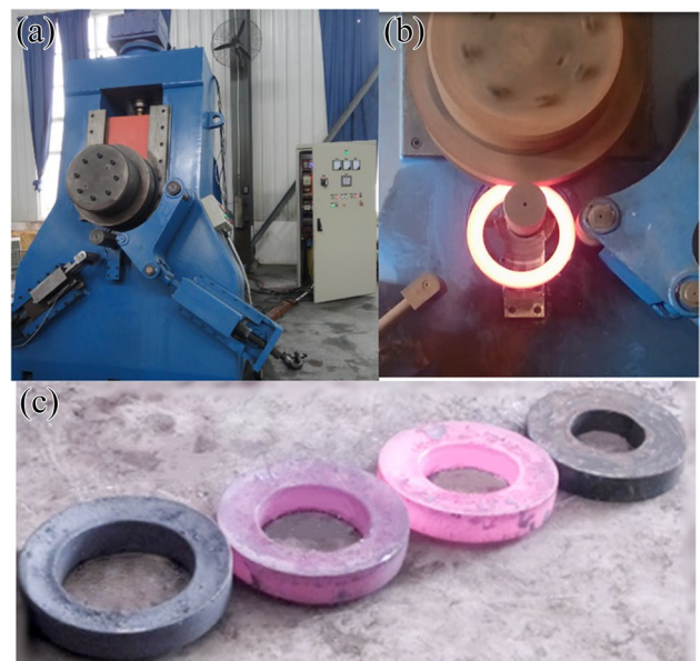
Fig. 4 HRR experiment of as-cast 100Cr6: a D51-350 NC HRR mill; b HRR process; c rolled rings under different deformation amount
