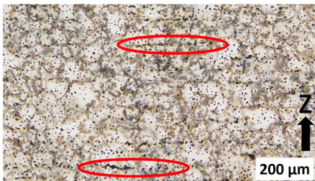
Fig. 12 Printing defects in FDMm sintered 1.2083 tool steel [83]
